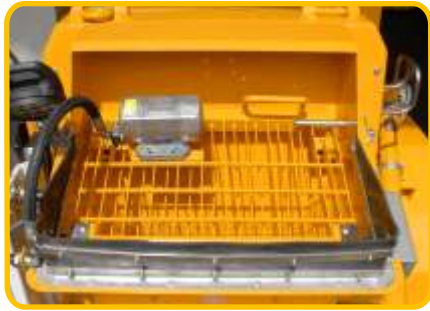
Specially designed hopper with agitator and vibrator grill for shotcrete operation with steel / polymer fibres.
